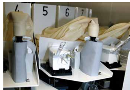
An attendant only needs to reload the daisywheel with radiosondes and balloons every 12 days.
