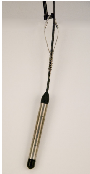
FIGURE 7-1. Transducer suspended with split mesh cable grip
