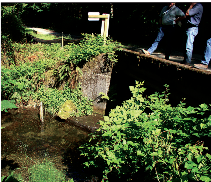
A turbidity sensor was installed in a tributary of the Cedar River watershed to monitor water quality conditions for Seattle, Washington.
