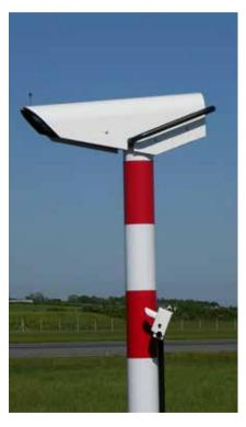
The Vaisala Background Luminance Sensor LM21 measures the ambient light level or background luminance in RVR applications. In the picture, the LM21 is installed on the Vaisala Transmissometer LT31.
